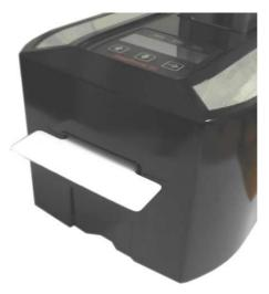
Picture 5: Cleaning card in cleaning position
