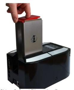
Picture 2: Insert "Hopper Load"
